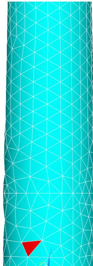
Figure (6.1) The damaged element, damage percentage and damage location of first scenario
