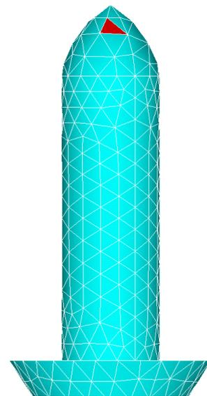
Figure (6.30) The damaged element, damage percentage and damage location of sixth scenario
